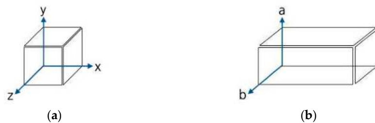
Figure 5. (a) Square for compressive strength test; (b) Rectangular for flexural strength test.
