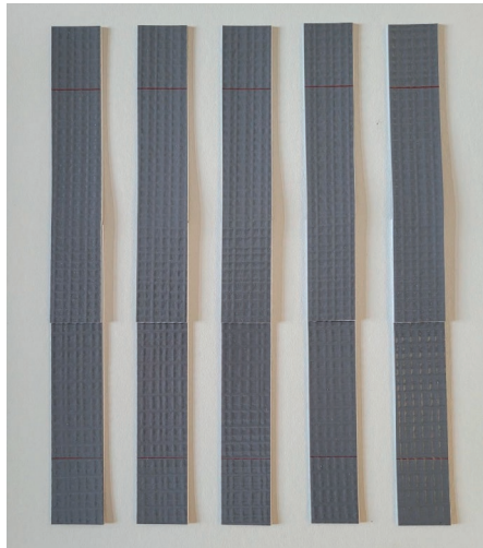
Figure 3. 5 samples for the tensile strength test of the material Bauder Thermofol U15.
