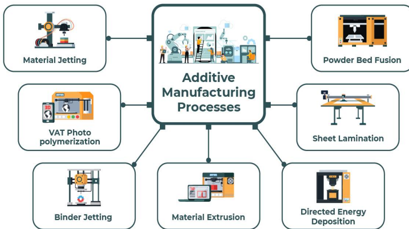
Figure 2.25: The seven main types of additive manufacturing processes [241].
