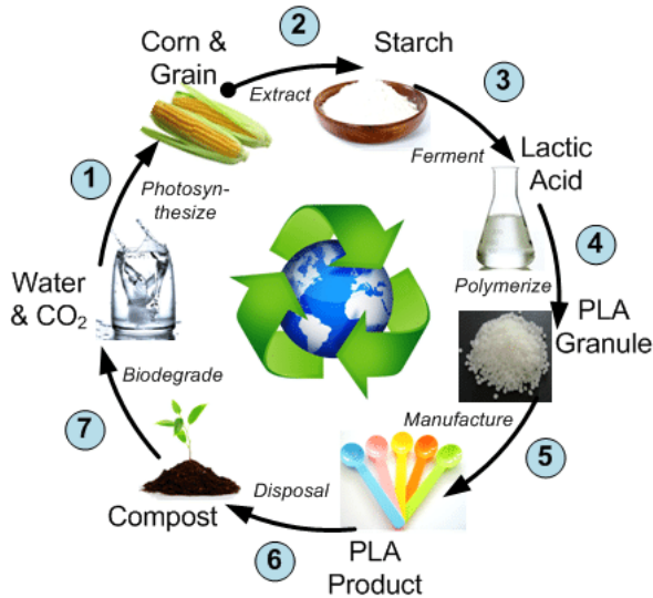
Figure 2.27: Diagram of polylactic acid (PLA) life cycle. Picture taken from Peng and Sun work [251].
