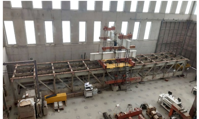
Figure 7. Complete span of a railway bridge inside the ICITECH laboratories.
