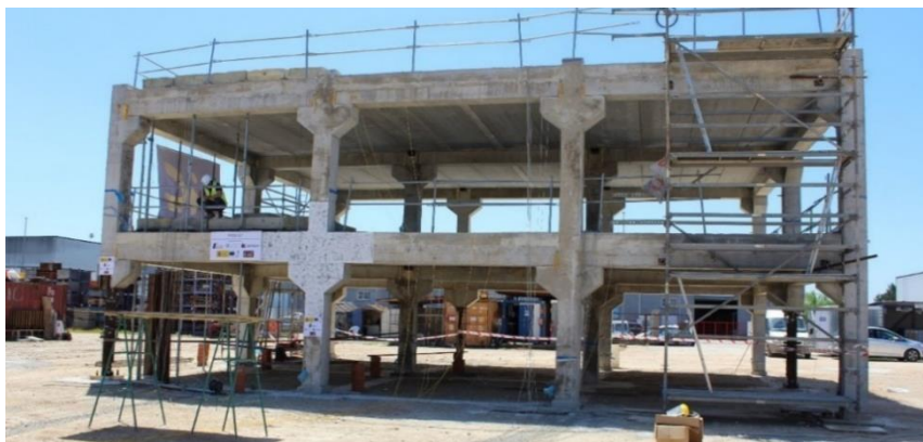
Figure 1. Completed building specimen prior to testing (Photo courtesy of Manuel Buitrago).
