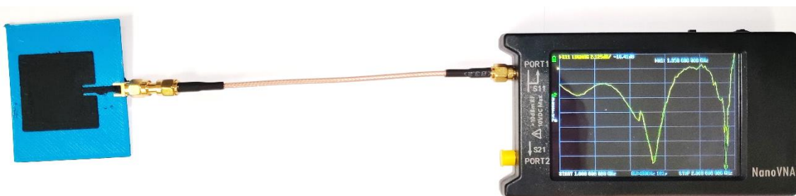
Figure 29: Antenna connected to VNA
