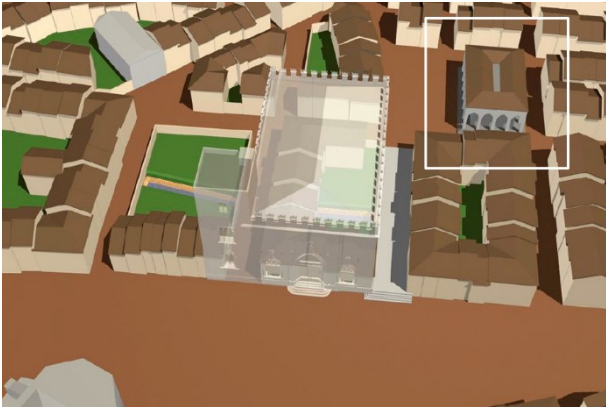
Figure 2: Graphic reconstruction of the Oil Market (Ramírez Blanco, 1999). The proposal of a perimeter porticoed structure can be appreciated as well as a central courtyard.
