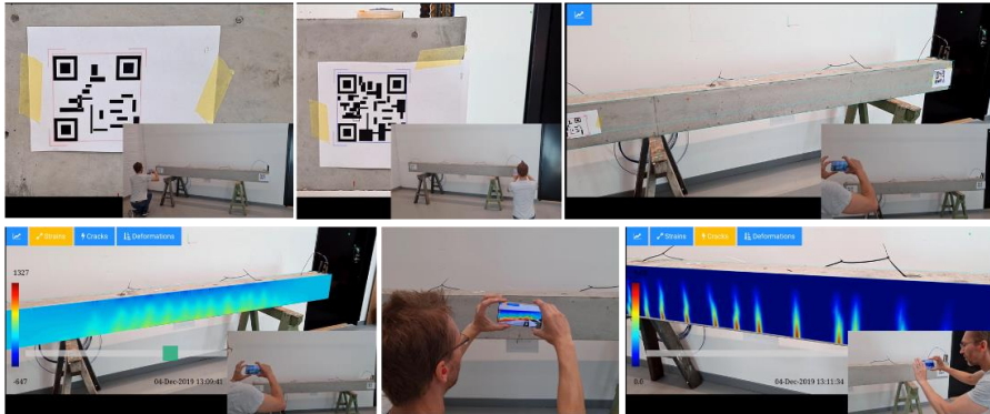
Figure 5. (a) Procedure to align the real and virtual beams in the AR tool using two markers. (b) The AR Tool interface ( https://youtu.be/y8yFHzpmzI8 )
