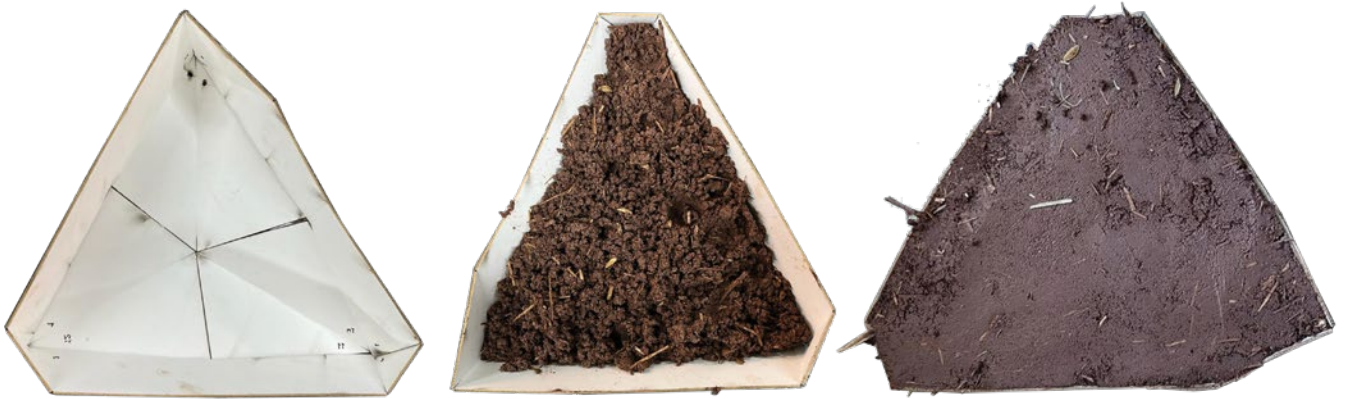
Figure 58_ Adobe mixture and the cardboard mold and adobe module imperfections (by author)
