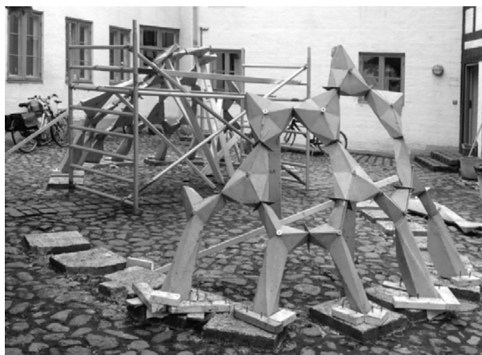
Figure 32_ Full-scale prototype assembly of external post-tension system (Beim and Madsen 2014; Pedersen and Larsen 2015)
