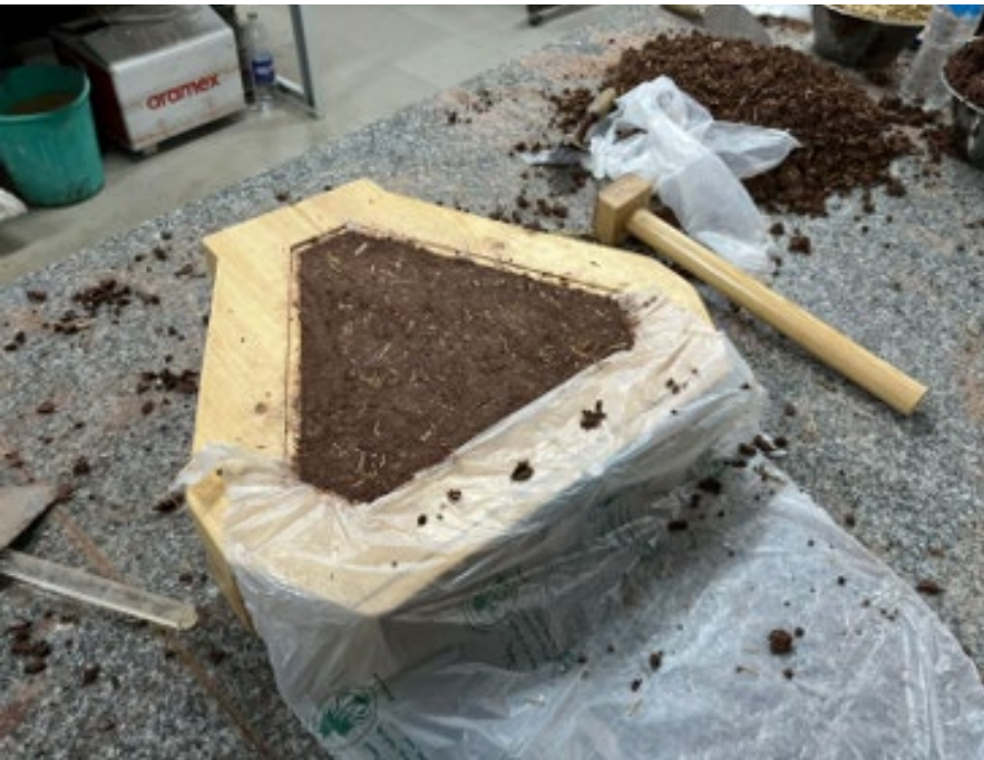
Figure 65_ specimens mixing, ramming and curing processes (by author)
