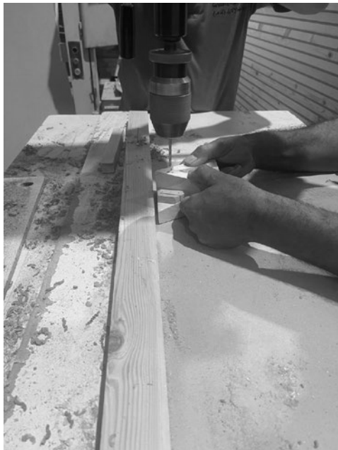
Figure 70_ Wooden connection and base fabrication (by author)
