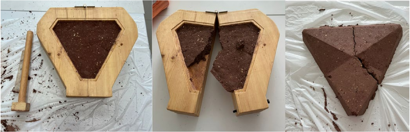
Figure 62_ Mixture adhesion to the mold causing cracks (by author)
