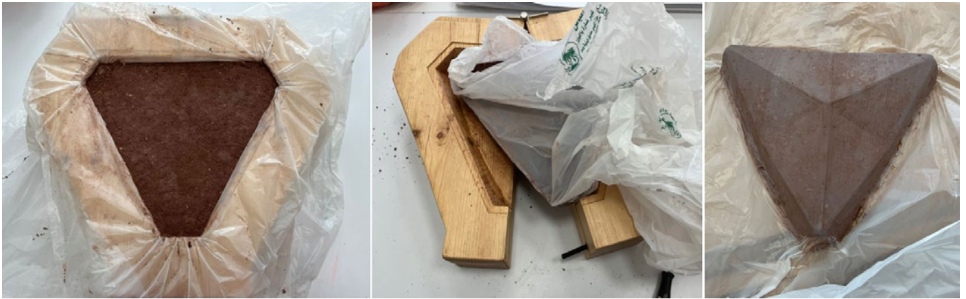
Figure 63_ CNC successful mold technique (by author)
