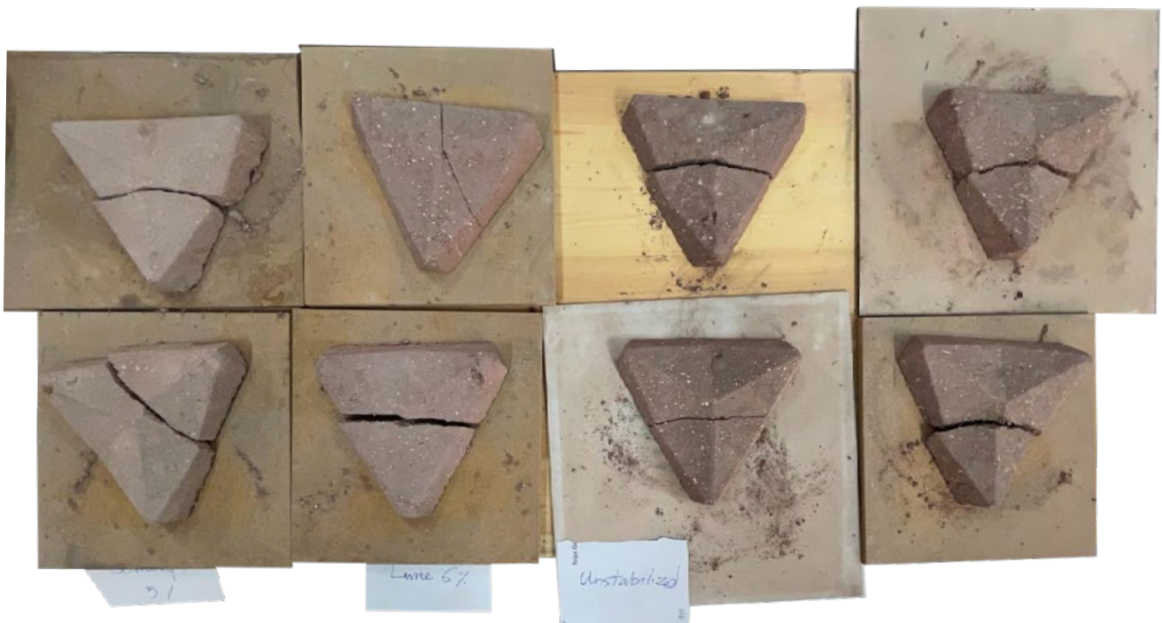
Figure 67_ Flexure test results (by author)
