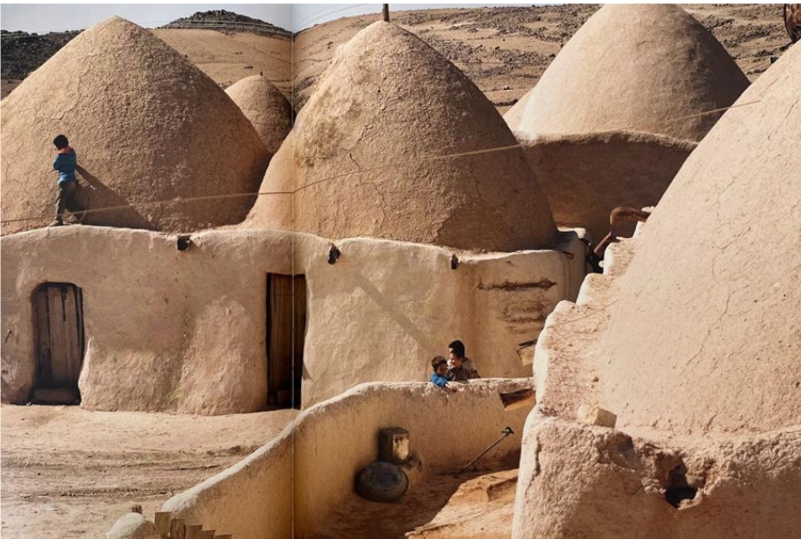
Figure 13_Beehive dome of mud with timber pieces for scaffold, Syria (Ragette 2003)
