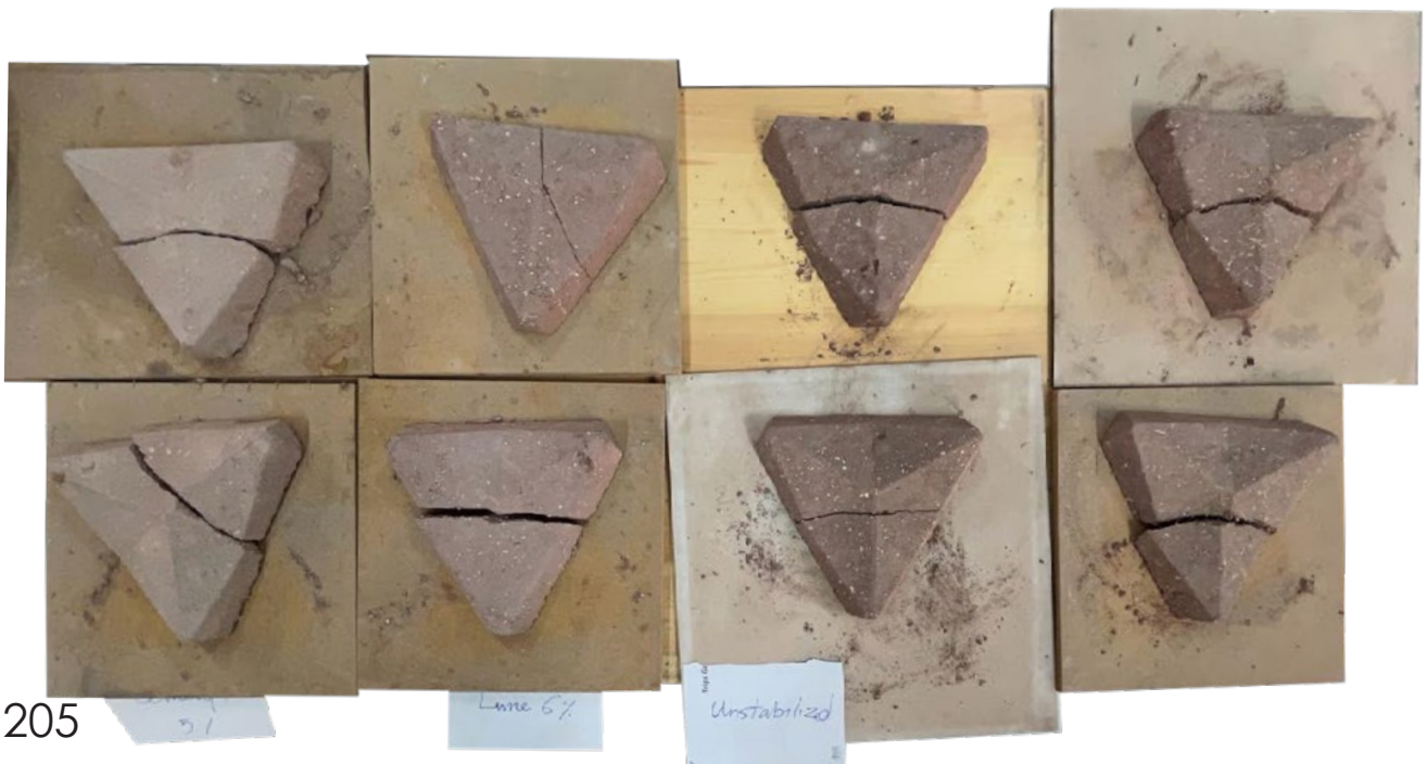
Figure 67_ Flexure test results (by author)
