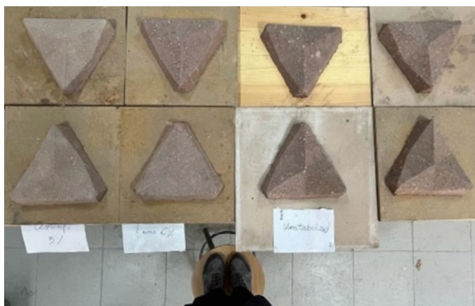
Figure 64_ Eight specimens for Flexure test (by author)
