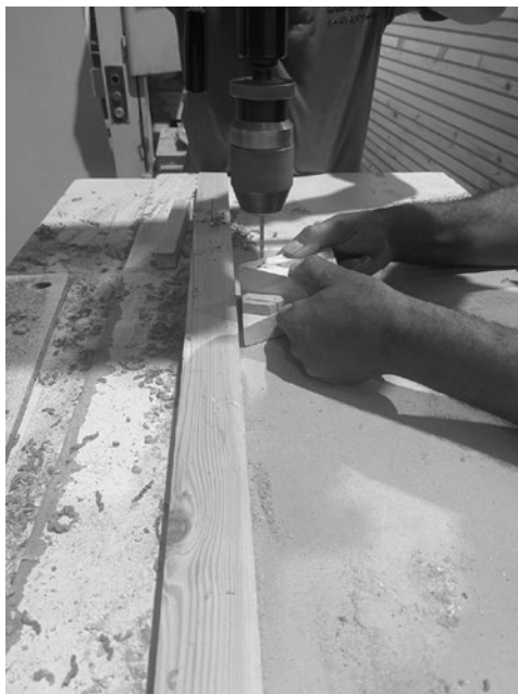
Figure 70_ Wooden connection and base fabrication (by author)
