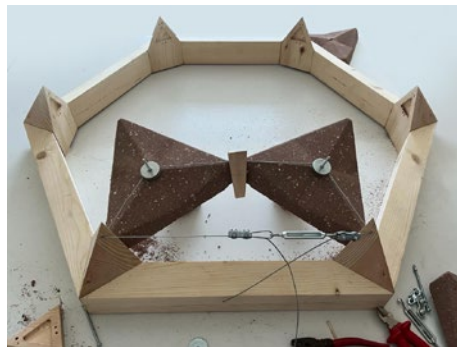
Figure 74_ Module corner thinning due to multiple fixation attempts (by author)
