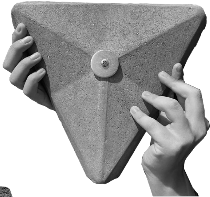
Figure 72_ Earth Module Detailing and hole drilling (by author)
