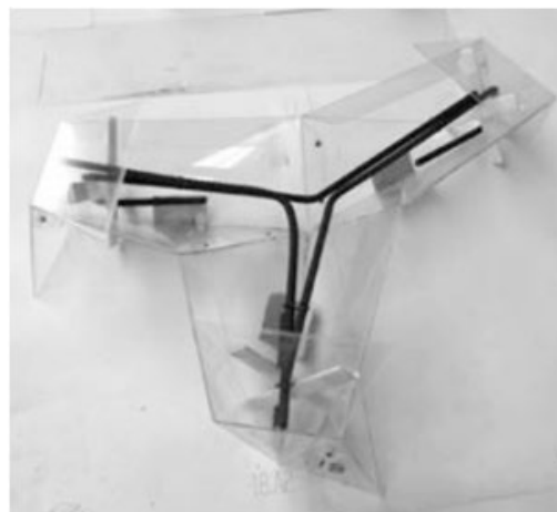
Figure 27_ Prototype of Y-shaped concrete component and template of PETG plastic (Larsen, Pedersen, and Pigram 2012)
