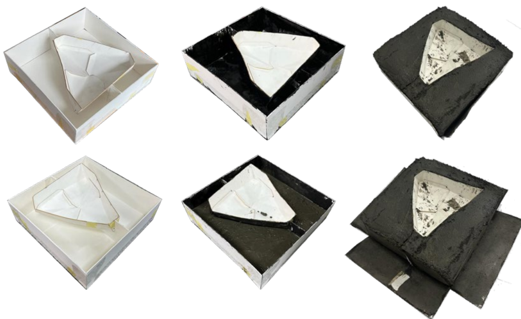
Figure 56_ Cement pouring in cardboard mould (by author)
