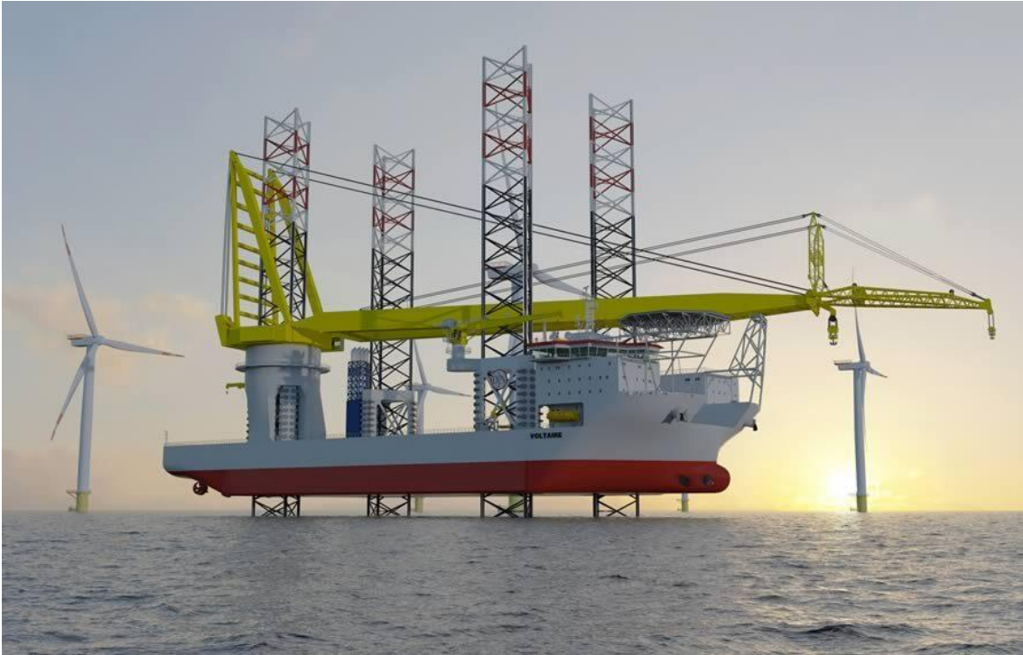
Fig. 8. Artist's impression of the new 'Voltaire' turbine installation vessel (Source: https://doggerbank.com/construction/ )
