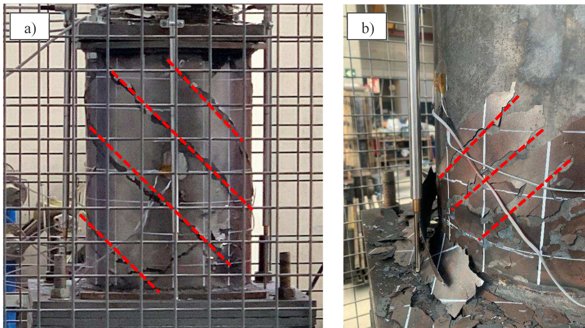
Fig. 10. Shear slippage lines: (a) SR-CFST-C-T1 during the test; (b) SR-CFST-C-T2 bottom end close up.
