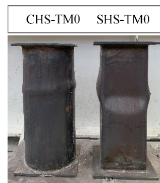
Fig. 12 Hollow columns after the tests
