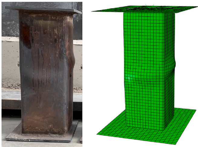
Fig. 8. Comparison between the experimental and numerical deformed shape for specimen SR-CFST-S-TM1.
