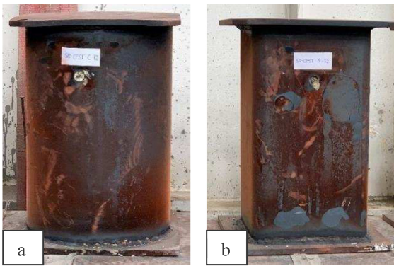
Fig. 7. External surface of the columns after heating: (a) SR-CFST-C-T2; (b) SR-CFST-S-T2.
