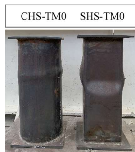
Figure 4.28 Hollow columns after the thermo-mechanical tests.
