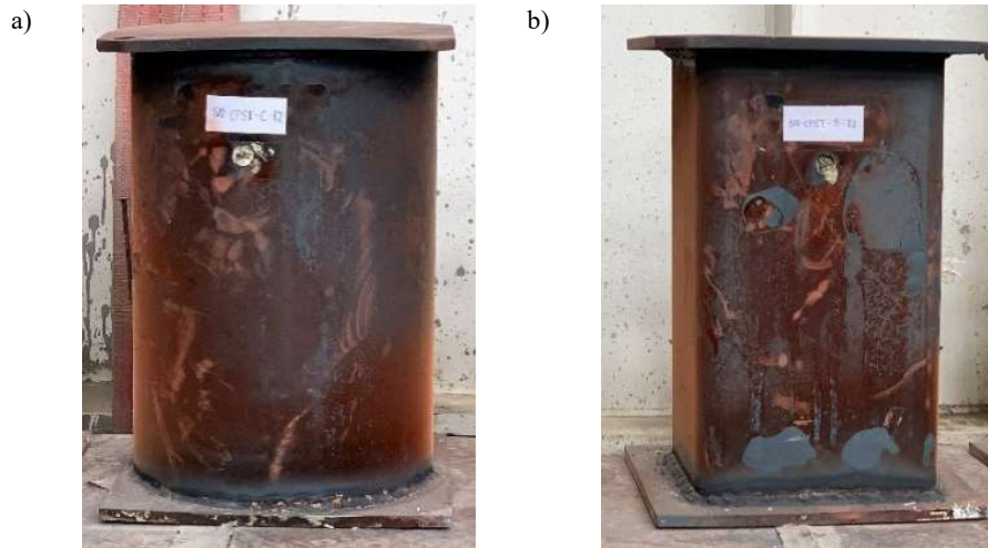
Figure 4.7 External surface of the columns after the heating tests: a) SR-CFST-C-T2; b) SR-CFST-S-T2.
