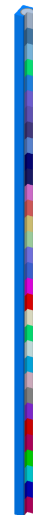
Figure 4.2: Single fuel rod representation in KENO3D displaying the 32 segments division (not to scale).
