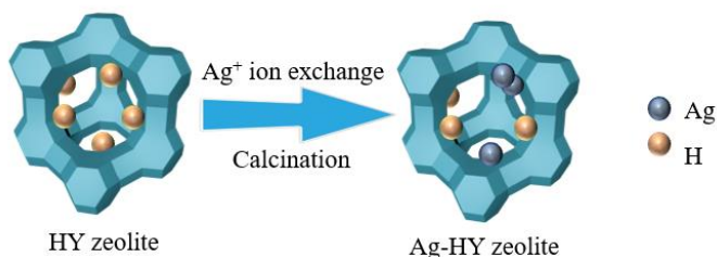
Figure 4.2 Schematic representation of the synthesis procedure of Ag-HY zeolites.
