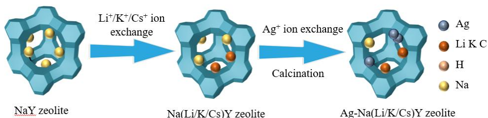
Figure 4.3 Schematic representation of the synthesis procedure of Ag-Na(Li/K/Cs) zeolites.
