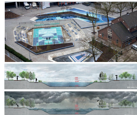
Figure 2.2.2: Example of temporary rainwater retention (source: Szymański, Szabra, Urbaniak, Gancarczyk, Sutkowska, & Sobieraj, 2023)
