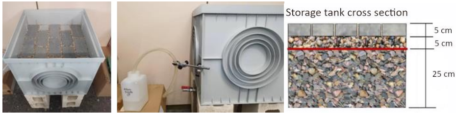
Figure V.2. Details of the storage tank setup and cross section. Geotextile is represented as horizontal red line. Own elaboration.
