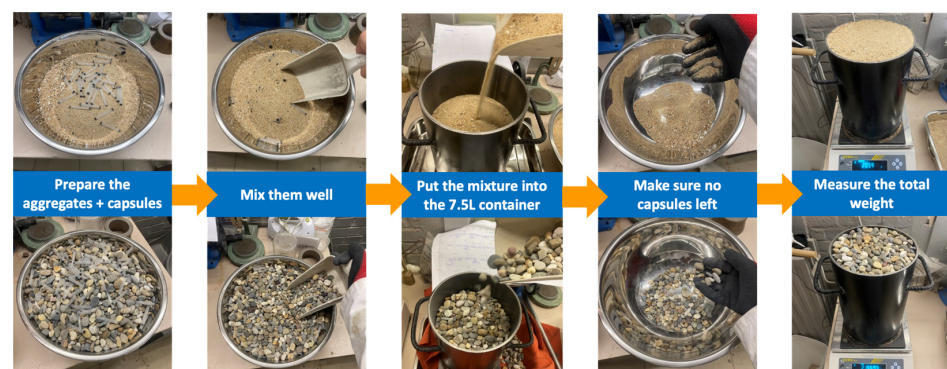
Figure 4. Schematic procedure of LBD test on a single type/fraction of aggregate.
