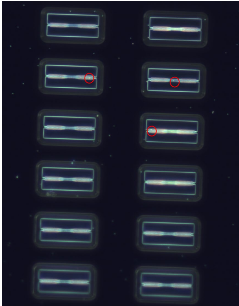
Figure 12: Optical image of an optomechanical cavities with Au NPs highlighted in red circles.
