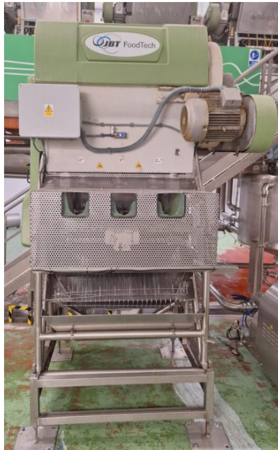
Figure 3. Photography of the JBT squeezer-type extractor used at Refresco Iberia for orange juice production.
