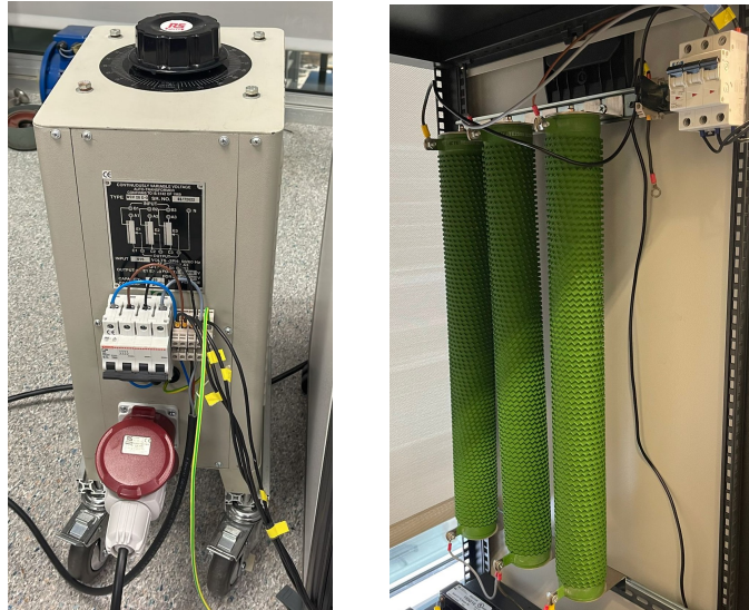
(a) Grid-connected auto-transformer.
