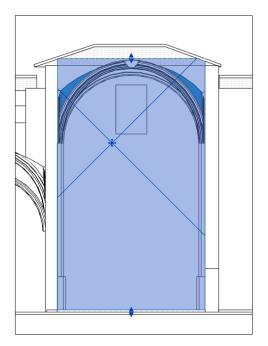
Figure 5. Volume of a room without vertical limitation visualised in a 2D section of Autodesk® Revit 2024. Source: Own elaboration (2024).
