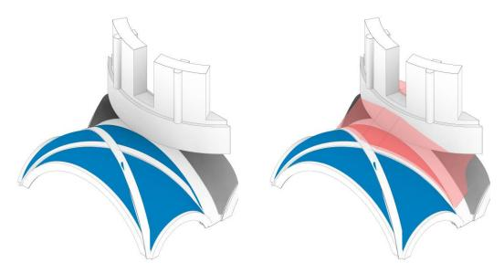
Figure 4. In blue - Modelling of the plementeries with the dough tool; In red - Error in the extrusion of the modelled plementeries. Source: Own elaboration (2024).
