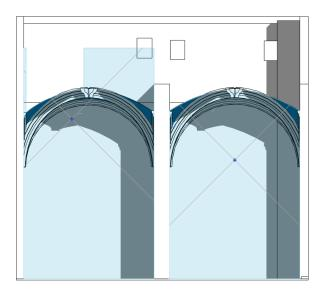
**Figure 6.** Volumes of two rooms constrained with the 'curtain wall' tool visualised in a 2D section of Autodesk® Revit 2024, (left) error in the vertical constraint, (right) vertical constraint corrected manually. Source: Own elaboration (2024).
