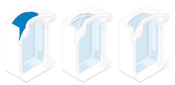
Figure 8. 3D volume vertically bounded by the de Autodesk<sup>®</sup> Revit 2024 "roof" tool visible by the Autodesk<sup>®</sup> plugin Dynamo. Source: Own elaboration (2024).
