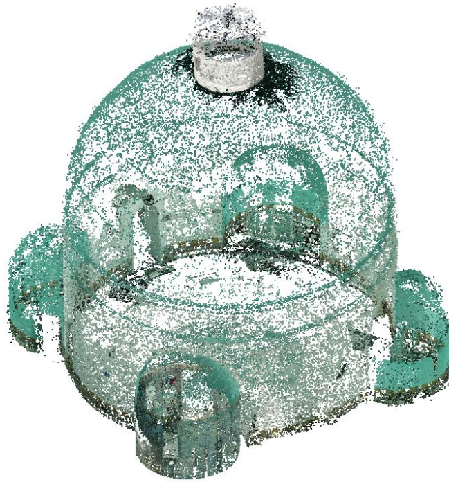
Figure 4. Point Cloud in Agisoft Metashape Professional of Cyan Dome Bath. Autor's work.
