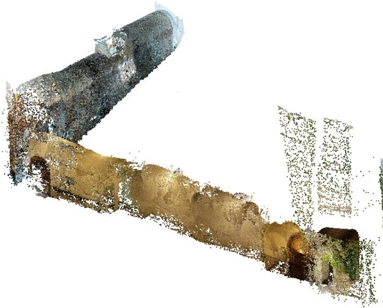
Figure 5. Point Cloud of Corridor and Stairs. Author's work.
