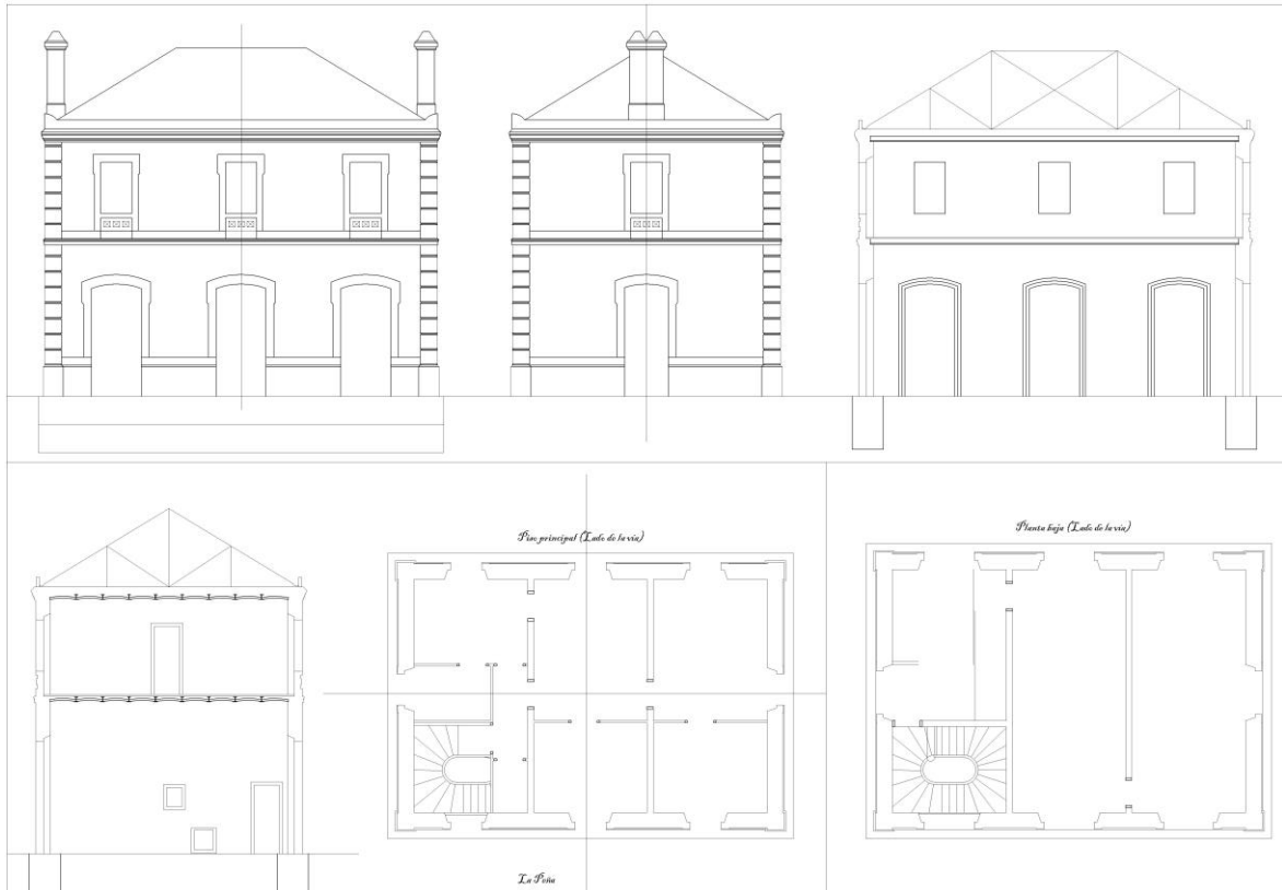
Figure 5. Floor Plans, Elevations, and Sections of the Passenger Building at La Peña Station. Source: Author.
