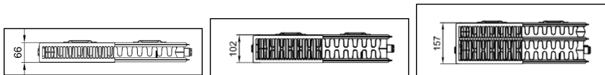
Figure 14: Top view and section of the radiators therm-x2 Plan-K type 12, 22 and 33 from Kermi GmbH (Kermi GmbH, 2024, p.23)
