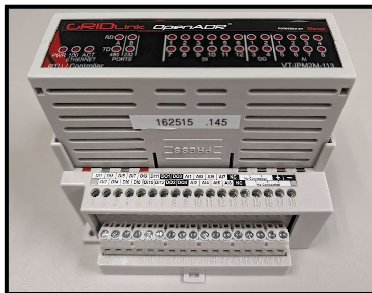
Figure 33: OpenADR hardware, GRIDlink series 113 inputs and outputs possibilities. Available at the e-SYM lab. Source: Own elaboration.
