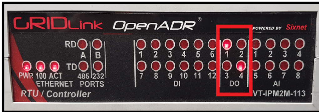
Figure 48: Hardware GRIDlink 113, digital output 1 is activated. Digital output 4 on means VTN connection is established. Source: Own elaboration
