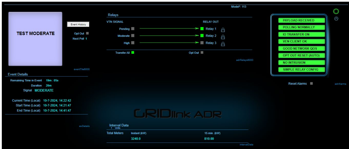
Figure 73: Simple signal with a moderate level – active phase. Relay 1 and Relay 2 is on. Source: Own elaboration
