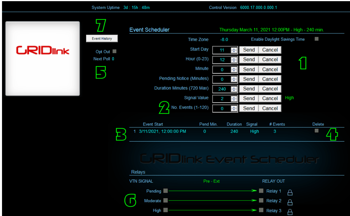
Figure 50: GRIDview overview for event scheduler. Source: GRIDlink Technologies [99]
