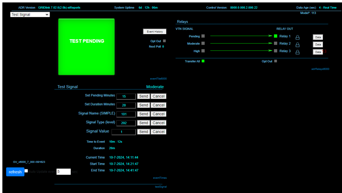
Figure 72: Simple signal with a moderate level – pending phase. Relay 1 is on. Source: Own elaboration
