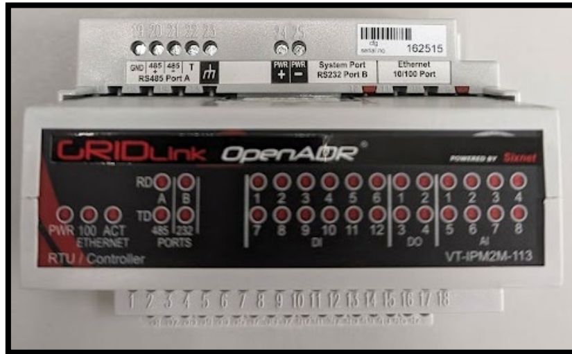
Figure 32: OpenADR hardware, GRIDlink series 113 front side. Available at the e-SYM lab. Source: Own elaboration.
