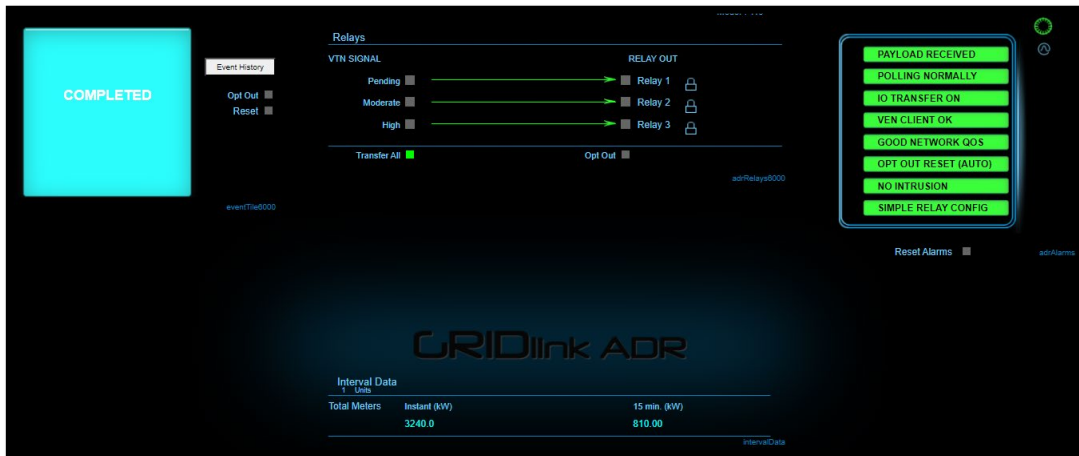
Figure 74: Simple signal with a moderate level – finished phase. Relay 1 and Relay 2 is off. Source: Own elaboration
