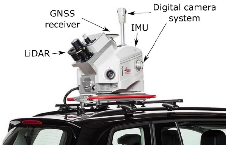
Figure 8: Example of an MMS: a vehicle-mounted mobile mapping platform consisting of different positioning and data collection sensors to generate an accurate georeferenced 3D map of the environment. [23]
