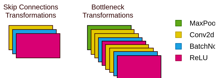
Figure 4.5: U-Net Transformations in the Skip and Bottleneck blocks.
