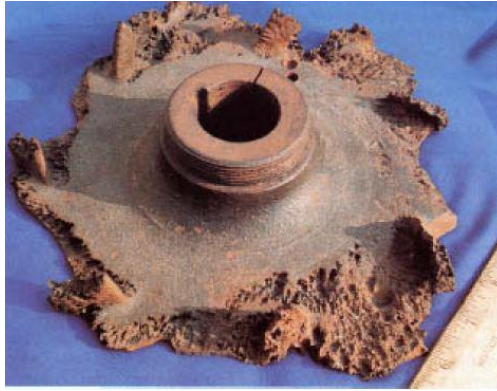
Figure 2.4. Part of a pump which has suffered cavitation.
