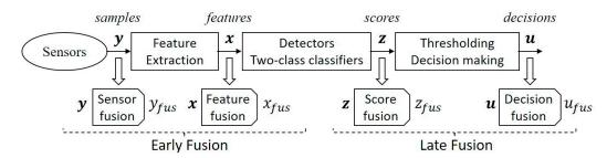
Figure 3. Outline of a data fusion pipeline in a detection system.
