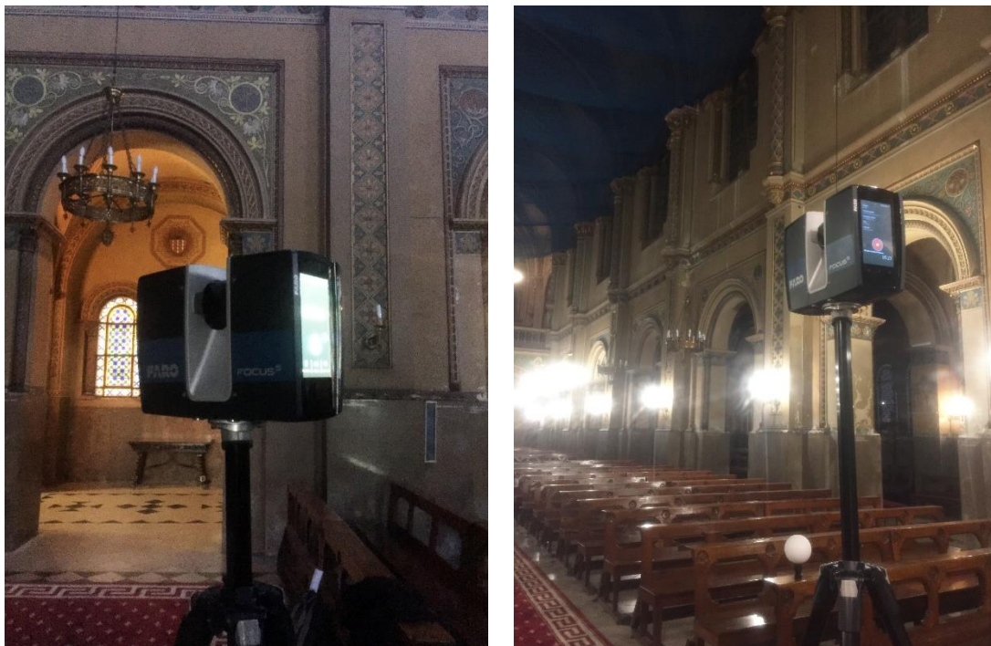
Figure 3. Faro Laser Scanner Focus 150 in the central nave.
