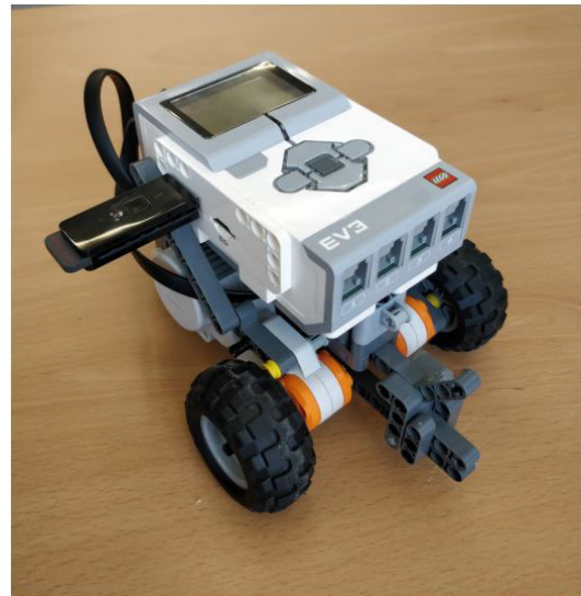
FIGURE 6. Two-wheeled mobile robot based on LEGO platform and Arduino.
