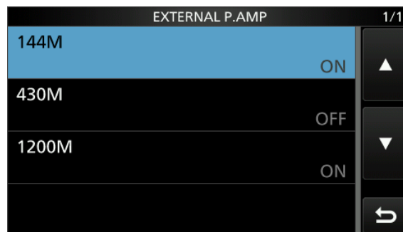
Figure 3.14 – ICOM-9700 external preamplifier supply settings per operative band (Menu > SET > Connectors > External P.AMP) [73].
