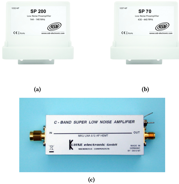
Figure 3.6 – VHF Low noise amplifier model [64] in (a), UHF Low noise amplifier model [65] in (b) and C-Band Low noise amplifier model for the transmission subsystem [66] in (c).
