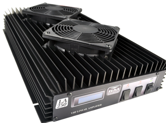
Figure 3.7 – Linear amplifier for the transmission subsystem [67].
