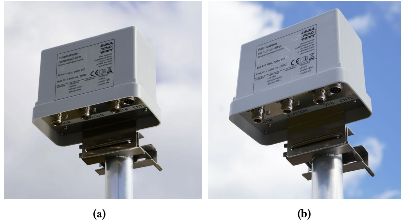
Figure 3.10 – Polarization switch models for VHF subsystem in (a) and for UHF subsystem in (b).
