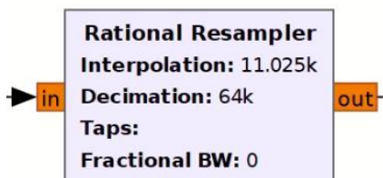
Figura 42. Bloque Rational Resampler.
