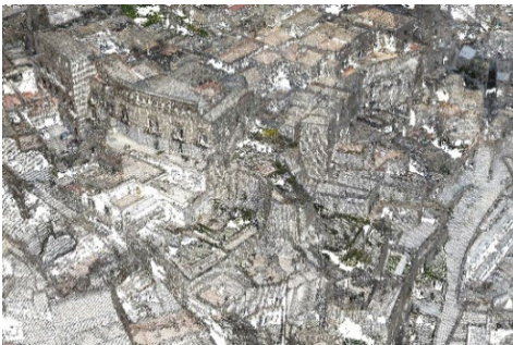
Fig. 3- Detail of the point cloud made with structure from motion techniques (Enrico Lamacchia, 2021)
