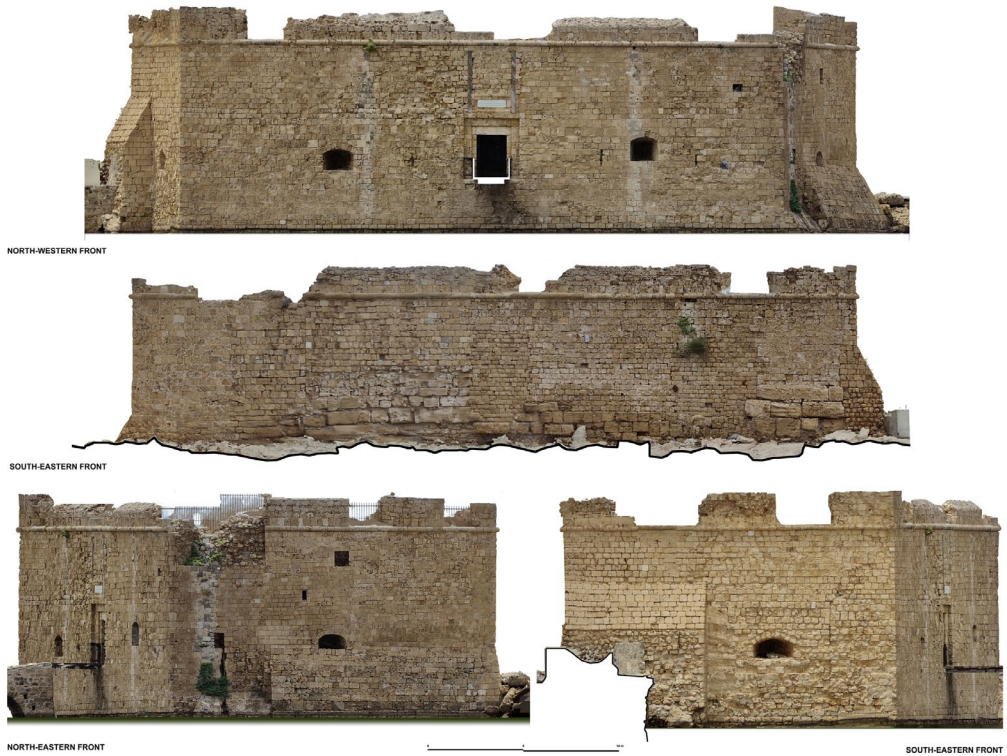
Fig. 6- The orthophotos obtained from the photogrammetry in June 2023 (photogrammetry and processing by the Authors).
