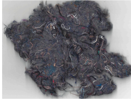
Figure 1. Visual aspect of the used textile waste from post-consumption of standard garments made with woven fabric.
