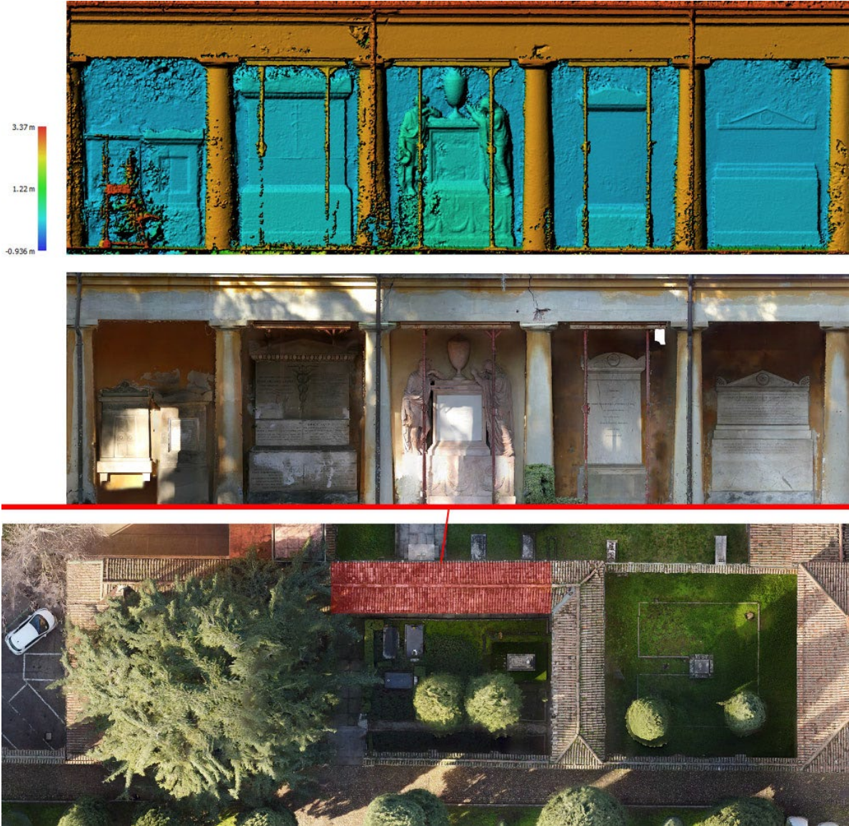
Fig. 6. Ground and drone orthophotos of the cloister and deep map extracted from the point cloud.
