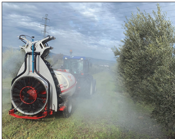
Figure 12. Validation of prescription maps with an air blast sprayer in traditional olive groves.
