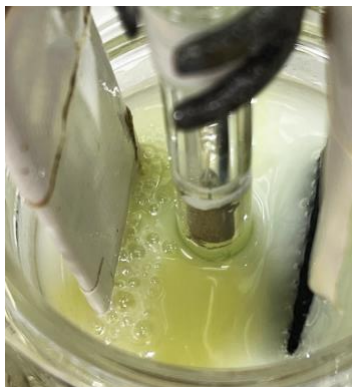
Figure 37: Formation and detachment of gas bubbles during (Galvanostatic) electrodeposition experiment.
