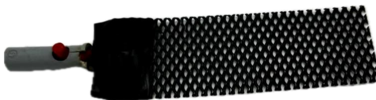
Figure 21: Mixed Metal Oxide - Mesh Counter Electrode, Dimensionally Stable Anode.
