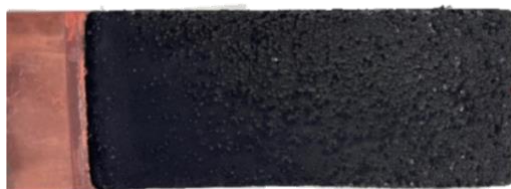
Figure 15: Previous work, potentiostatic electrodeposition at a current density of 1.875 \text{ mA}\cdot\text{cm}^{-2} for a duration of 120 min.
