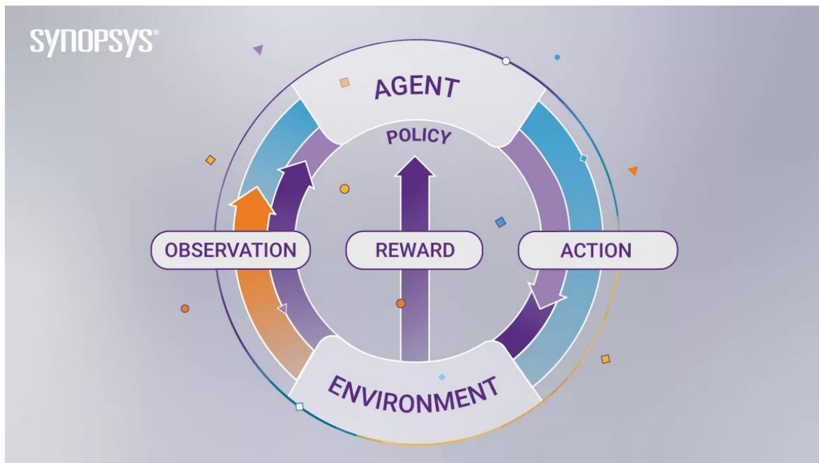
Image 8. Diagram of how Reinforcement Learning works. (Synopsis 2021)
