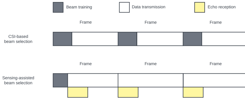
FIGURE 5. Frame structure in a DL transmission.
