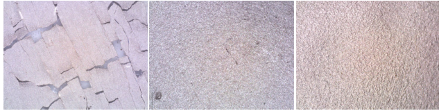
FIGURE 9. SEM images (100 times magnification) of the ink printed in PDMS (left), PDMS with plasma treatment (center) and PMA (right).
