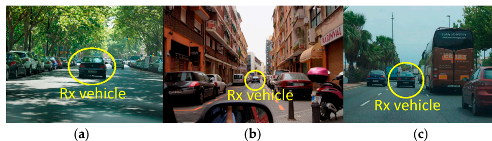
Figure 5. Measurement scenarios, (a) urban high density, (b) urban low density, and (c) suburban. The Rx vehicle can be seen driving in front of the Tx vehicle.
