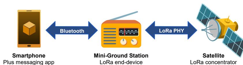
Figure 1.4 – Simplified schematic of the devices and protocols involved in the users' segment.
