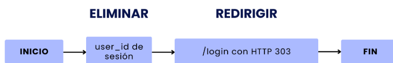
Figura 75. Diagrama de flujo endpoint POST logout
