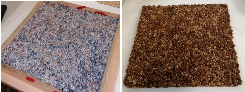
Fig. 3. A) Mixture in the mould. B) Dried board.
