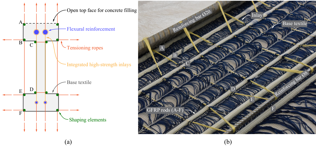
FIGURE 1 Thin-walled concrete beams from folded textiles: (a) cross section (in upside-down casting position); (b) flat textiles before tensioning with integrated flexural and textile reinforcement, and shaping elements.
