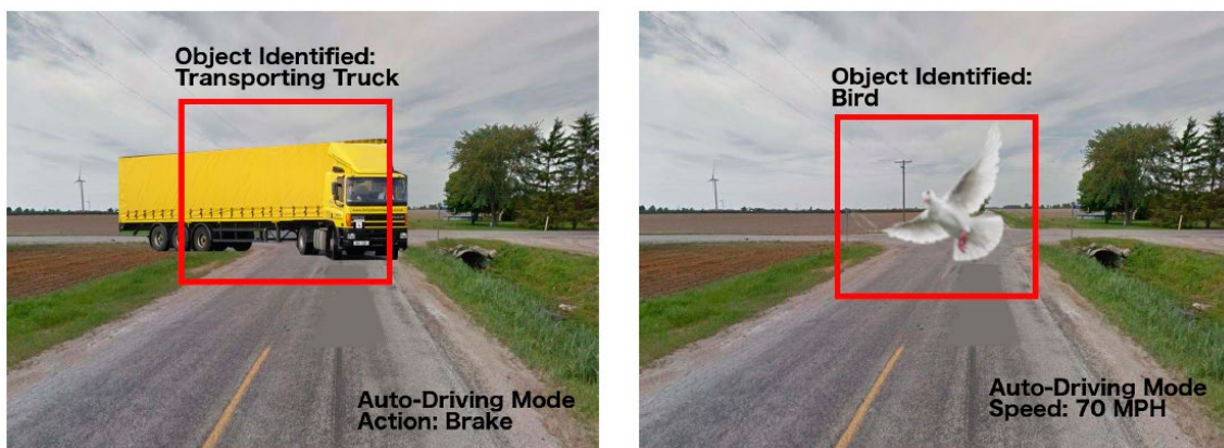
Figure 1. Example of SDC that could lead to collision in self-driving cars due to soft errors: (left) Fault-free execution and (right) SDC.
