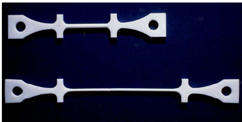
Figure 1. 3YTZP deformed at 1450 °C and 3 \times 10^{-4} \text{ s}^{-1} (Courtesy to Prof. F. Wakai)
