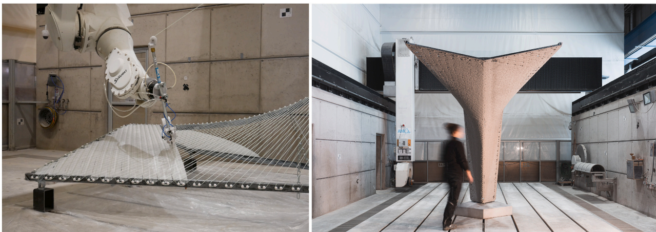
Fig. 17. Frame fibre winding process with visible white layer of mesh deposited simultaneously with the second layer of fibre yarn (left), and finished demonstrator with concrete applied through spraying (right); ©ITE, TU Braunschweig.
